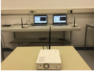
Figure 2. Lab measurement setup consisting of three Ettus USRP devices.
